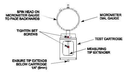
Figure 3-17. Setting Up Tools from Height Gauge Kit.
